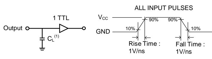
1. Including jig and scope capacitance.
